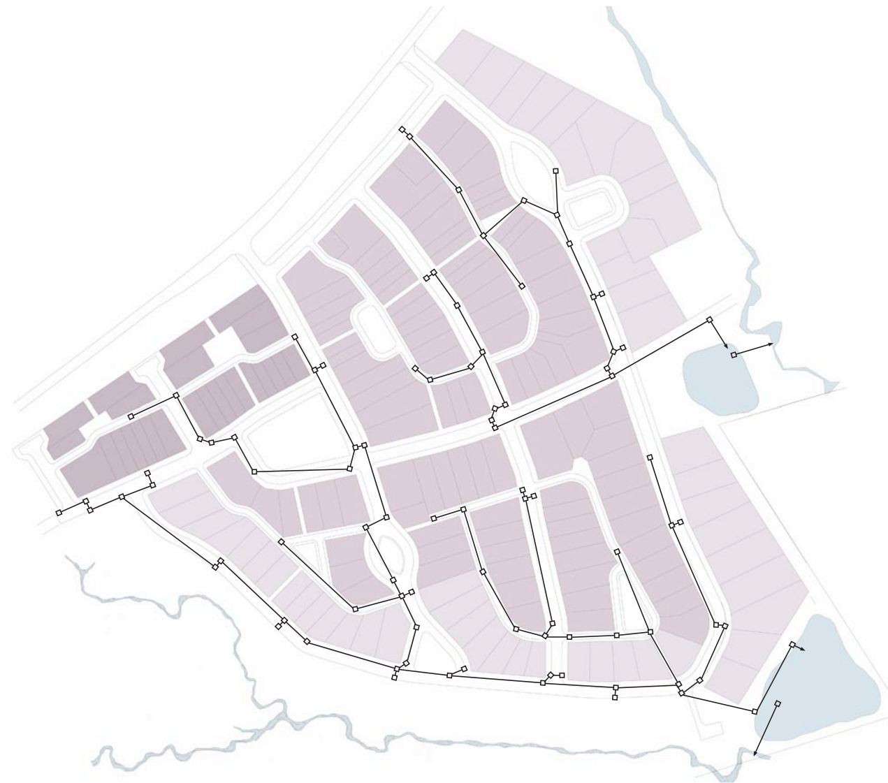
CONVENTIONAL TND STORM WATER PLAN
